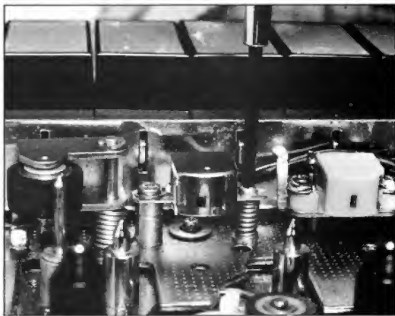
Figure IV: A close up view of the azimuth adjusting screw next to the record/play head
